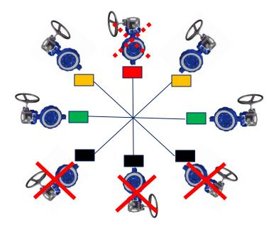
In case of installation with actuators, take into account the recommendations of the motorized accessories manufacturers (breaking risk of the lubricating function in some positions).
